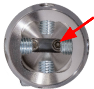
Fig. 1: Loosen and remove the screw that will allow the direction of slide. Do not remove other screw! For example, remove left screw to slide to the right.
